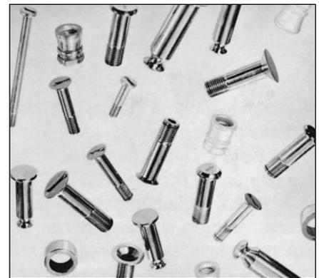
Figure 7 **WHEN COLD WORKING IS EMPLOYED, SOME NORMALLY NON-MAGNETIC AUSTENITIC STEELS BECOME SUBSTANTIALLY MAGNETIC**
