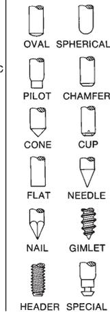
An analysis of standard fasteners, such as bolts and screws, reveals that all have certain characteristics in common. Further, their differences can be classified as shown here. Each bolt and screw is, in effect, made up of a series of component parts; thus, the fasteners may have some or all of these: (a) a head; (b) a driving recess; (c) a shoulder; (d) an unthreaded shank; (e) a threaded shank; and (f) a point.
