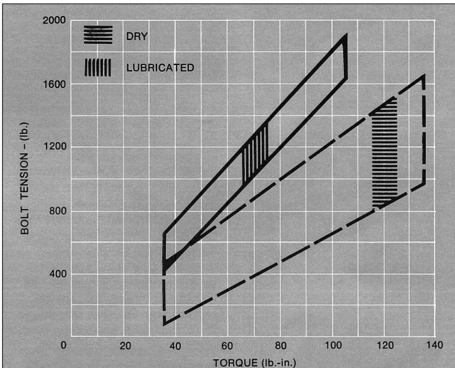
Effect of lubrication on torque-tension relationships is shown by the chart which is based on results obtained with 9/16-18 steel bolt driven into aluminum. For a non-lubricated bolt, torques of 115 to 125 lb.-in. were required to develop tensions of 800 to 1400 lb. For a lubricated bolt, torque values ranged from 65 to 75 lb.-in. for 1000
