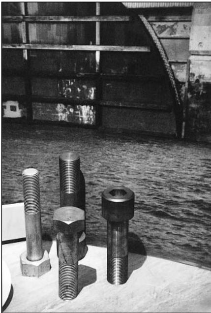
Typical stainless steel structural bolting.
