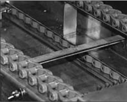
Stainless angles were used to construct a Bar Screen (Series 1000 from Envirex, INC) for a water treatment application.
