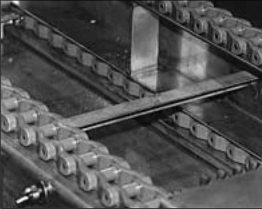
Stainless angles were used to construct a Bar Screen (Series 1000 from Envirex, INC) for a water treatment application.
