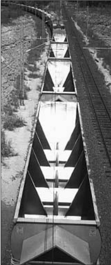
Rail coal carriers fabricated from stainless steel.
